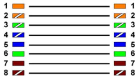
The other cable is called a straight through cable, and as the description says it's a cable scheme where the color-coded wires are the same on both sides of the connector. There are different wiring schemes, and standards but functionality wise it shouldn't matter as long as you follow the proper cable scheme for connecting to the type of device you're using.
