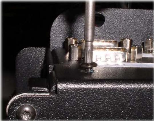
After locking the card into place you should double check it to make sure the card is seated, and that nothing is shorted out. Once you're absolutely sure put the other three screws on this side back on, then the three on the bottom, and finally the one other screw pictured to your left.
