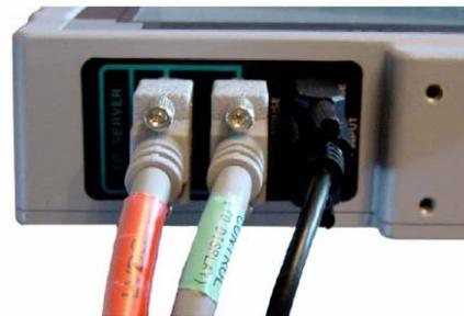
1. Connect the keyboard to the black LCD connector labeled **PS/2 KEYB/MOUSE INPUT**.
