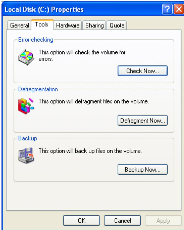
The first step is your scan disk, and clicking the “Check Now” button under Error-checking will launch this tool.
