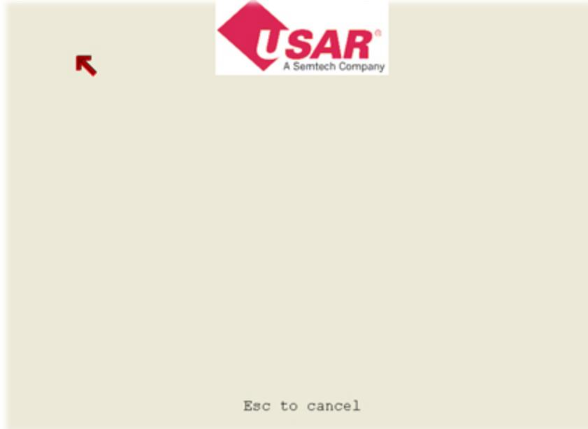
Using your finger or stylus touch the tip of the arrow shown on the screen, and then move on to the next point. You will have to touch the arrow in all four corners before your touch screen is properly calibrated.
