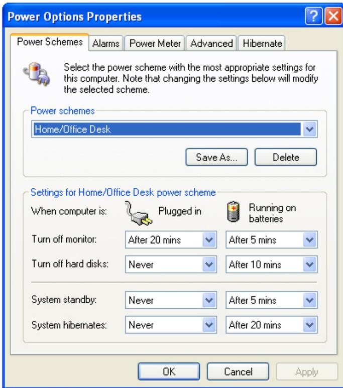
This window should be relatively self-explanatory. It allows you to set power management modes for when plugged in to a power source, or when you're running a battery through the Smart UPS port.
